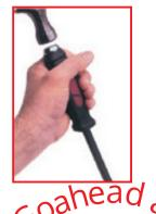
Capped end in direct contact with shaft.
